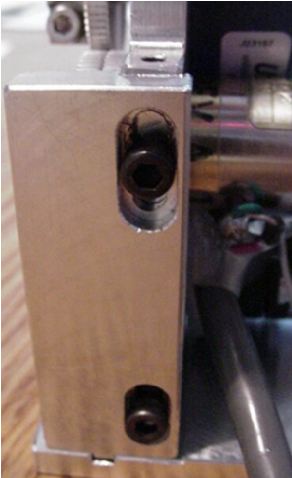
Figure 6: Loosen but do not remove adjustment screws
