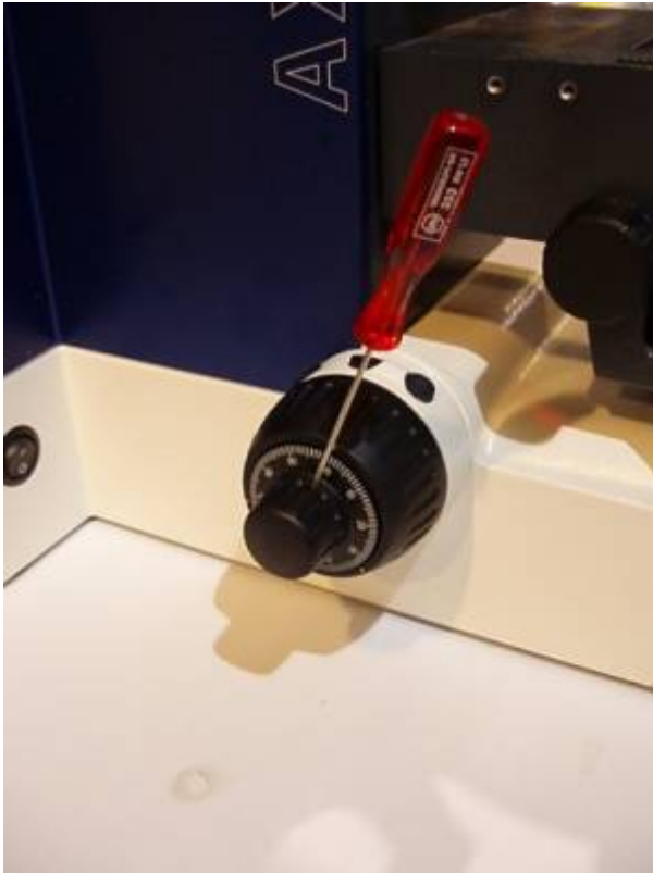
Use 1.5 mm Allen wrench to loosen set screw.
