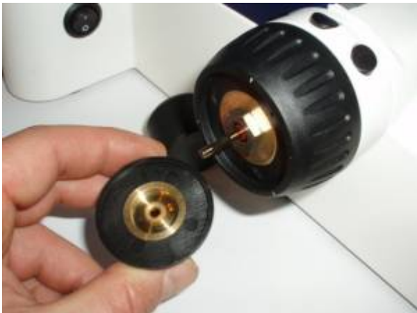
Pull knob straight off to expose shaft
