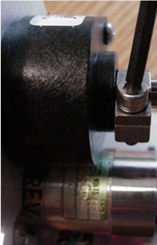
Figure 7: Tightening the drive shaft clamp.
