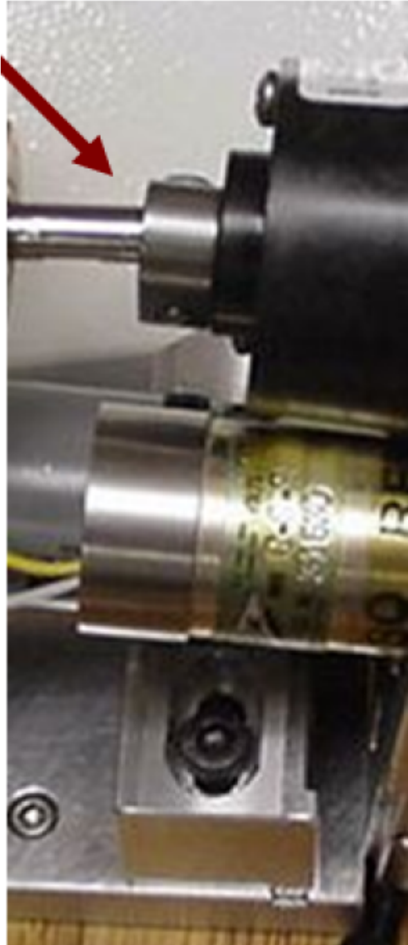
Figure 5: Slide ASI drive shaft onto microscope's fine focus shaft.
