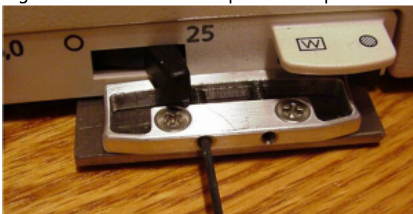
Figure 8: Install the baseplate clamp between the switches.
