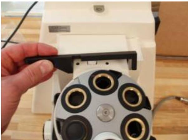
Figure 1. Linear encoder mounted on Axiovert
