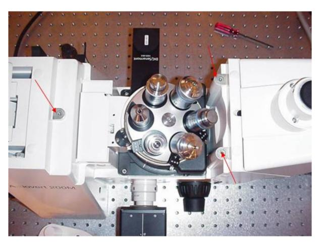
Location of three 4 x 12 mm screws that secure stage to Axiovert /AxioObserver. There are two in the front & one in rear. Use 3mm Allen wrench to remove screws & then remove stage.
