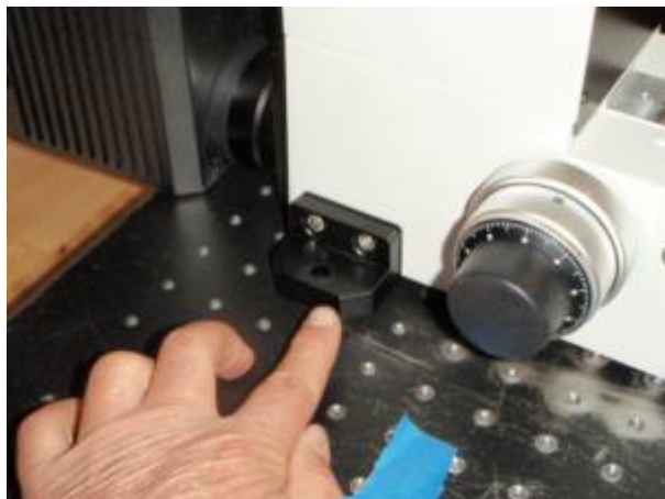
Figure 2. Standard Nikon adapter plates mount onto the microscope body at four points. Please refer to the Nikon manual for information on mount these plates
