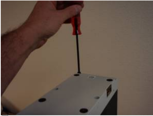
Figure 7. Location of four screws that remove / secure trinocular head base
