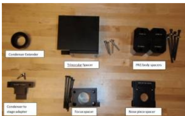
Figure 1. Spacer and adapter kit to adapt ASI FTP-2100 stage to Nikon FN1
