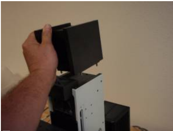
Figure 8. Installing the trinocular spacer, note alignment pins
