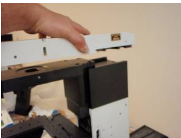
Figure 11a. Installing the trinocular mount back onto the microscope body
