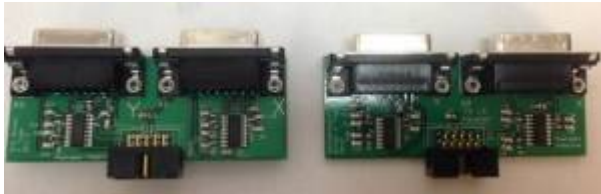
Figure 1: Linear Encoder Buffer card, Left card is for MicroE and Renishaw. Right is for Heidenhain
