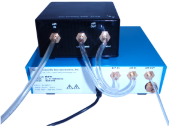
Rear view of MPPI-3 connected to BPU
