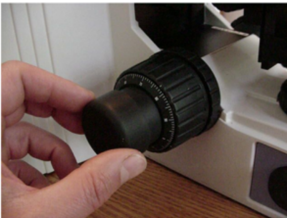
Figure 1: Pull off rubber boot
