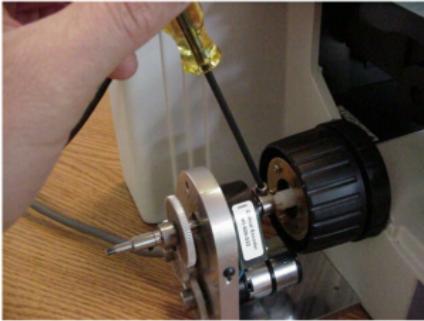
Figure 10: Tightening the drive shaft clamp
