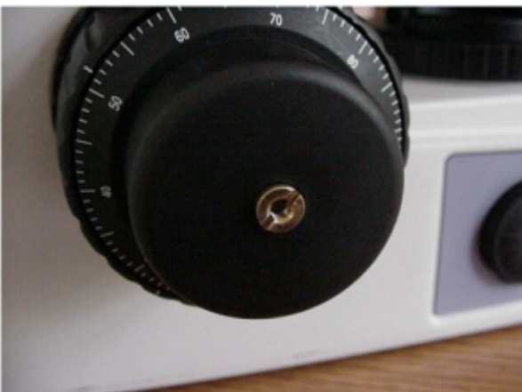
Figure 2: Use screwdriver to remove nut
