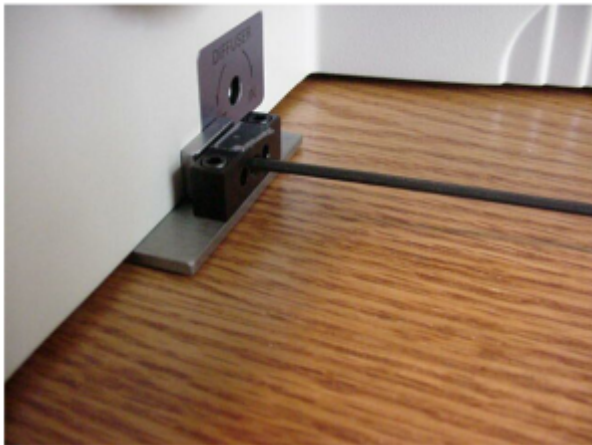
Figure 9: Tighten baseplate clamp after drive is installed & roughly aligned
