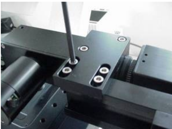
Fig 4a: Perpendicular adjustment bracket (tool needed 9/64" hex wrench)
