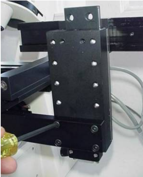
Fig 3c: attach LS50 to mounting bar
