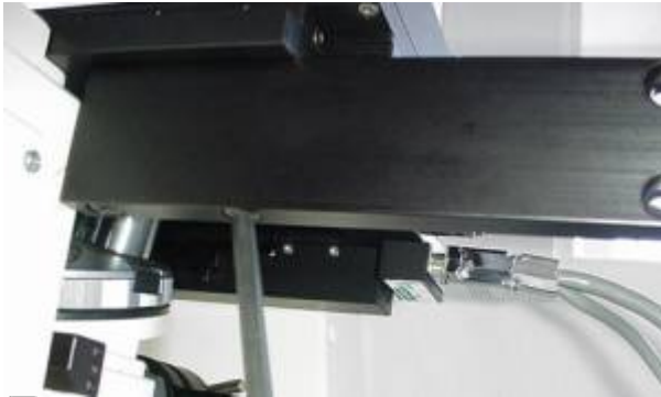
Fig 3a: Install Bar to stage
