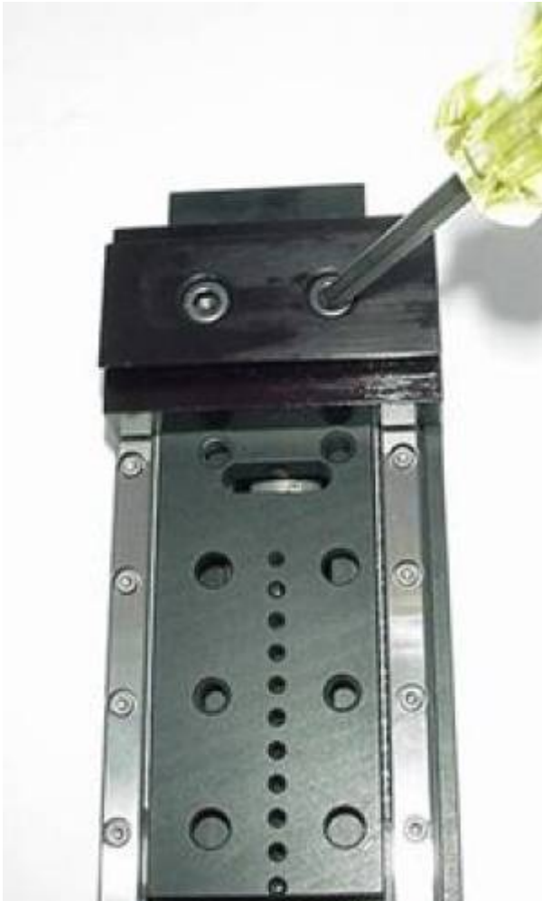
Fig 3b: attach male dovetail to LS50
