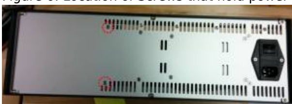
Figure 7: Location of Screws that hold power supply on Back panel in a TG-16 controller
