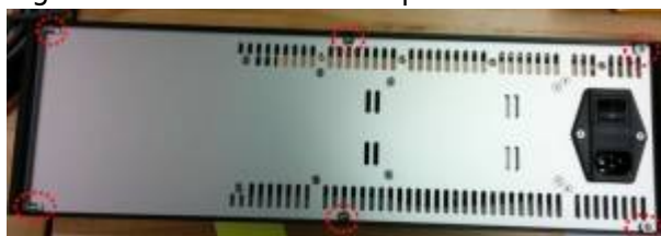
Figure 3: Location on Back panel screws on a TG-16 controller
