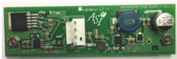
Figure 1: 5 volt Power supply used in TG controllers
