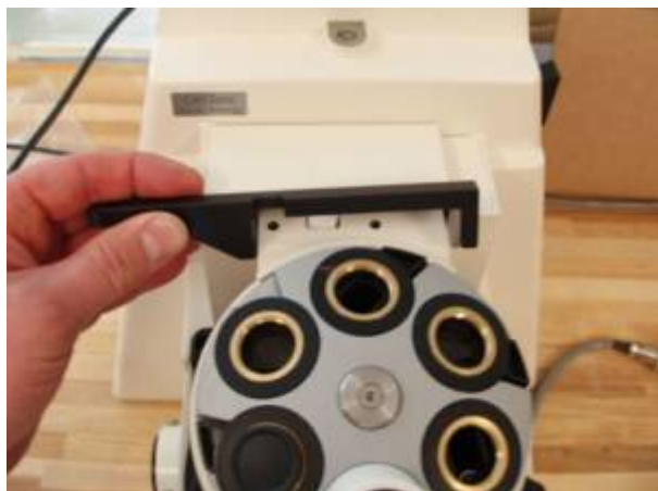
Figure 1. Linear encoder mounted on Axiovert
